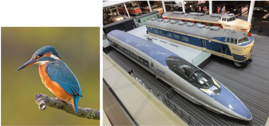
Fig. 4 The common kingfisher bird's bill inspired the high-speed train's nose [28, 29]
